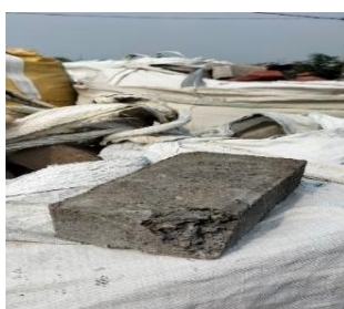
Gambar 3. Defect Gupil (sumber: PT. Pesona Arnos Beton)
