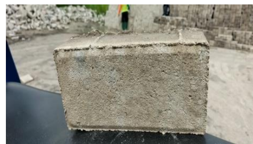
Gambar 2. Defect Presisi (sumber: PT. Pesona Arnos Beton)
